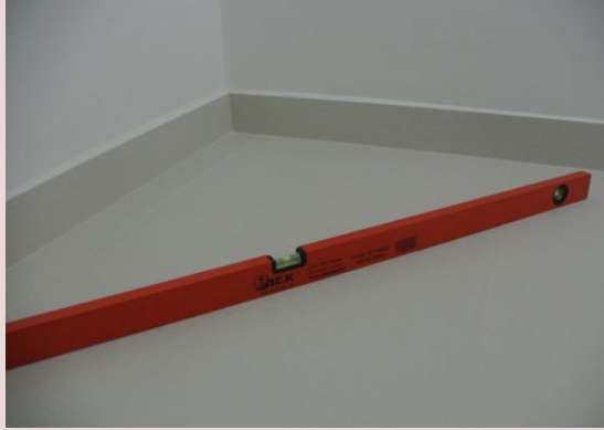
Evenness not more than 3mm over 1.2m Figure 5.5.i
