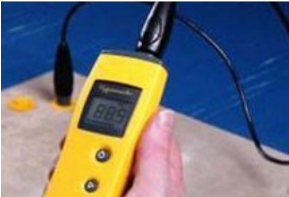
Checking of RH by drilling Figure 4.2.2.a
