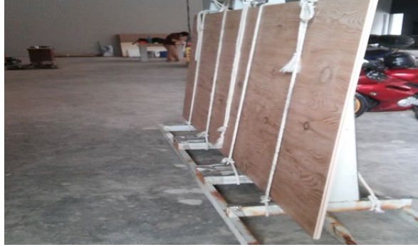
Handling and transport using A frame
